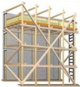
Double Pole Scaffold
